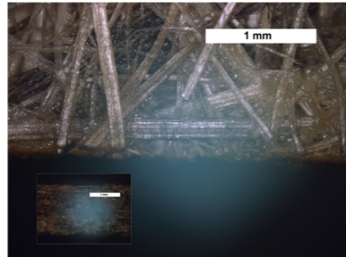
Cutting of organic compound 1.5 mm thick Speed: 1.2 m / min (wood/resin)
